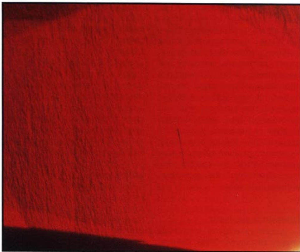
Figure 7— Needle-like inclusion in a hydrothermal synthetic ruby following the striated direction of the graining pattern. Photomicrograph, immersion, 40X.
