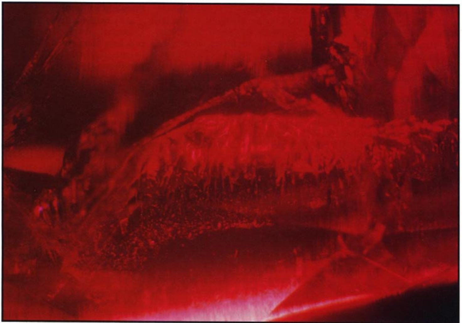
Figure 8— Healed fracture systems present in a hydrothermal synthetic ruby. These fingerprint-like inclusions occasionally contain gas phases. They are transparent and colorless and may potentially be confused with healed fracture systems of natural rubies. Photomicrograph 35X.
